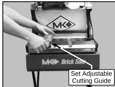
(B) Set the Adjustable Cutting Guide to cut a 1/16-strip
