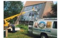
**Boom Lift - Trailer** The trailer-mounted boom lift provides 42' of working height and 32' of outreach and features an automatic, self-leveling hydraulic outrigger system that allows for setup in 30 seconds when all four outriggers are deployed simultaneously.
