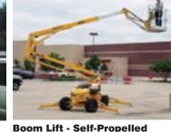
**Boom Lift - Self-Propelled** Our self propelled boom lift features a hydraulic lift system with industry-leading leveling capability that allows you to set up and begin operation in under 30 seconds. Our self propelled boom lift gives you a working height of 51' and a horizontal outreach of 27'. Scissor Lift Our compact scisso
